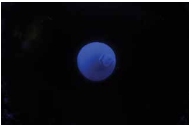
Figure 14: When exposed to long- or short-wave UV radiation, the glue used to affix the HoP tag in this prototype example fluoresces blue, while the surrounding cultured pearl is inert, enabling the marker to be easily located. The size of the fluorescent spot is approximately 1 mm in diameter. Photomicrograph by O. Segura.
